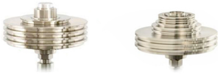
MP and MGP measuring deadweight tester systems with load sets
